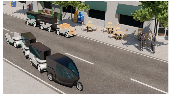
Fig. 1. A Ducktrain of three Follow-Me Ducks following a passenger micro vehicle (front) and another Ducktrain of three parked at the side of the road (back).
