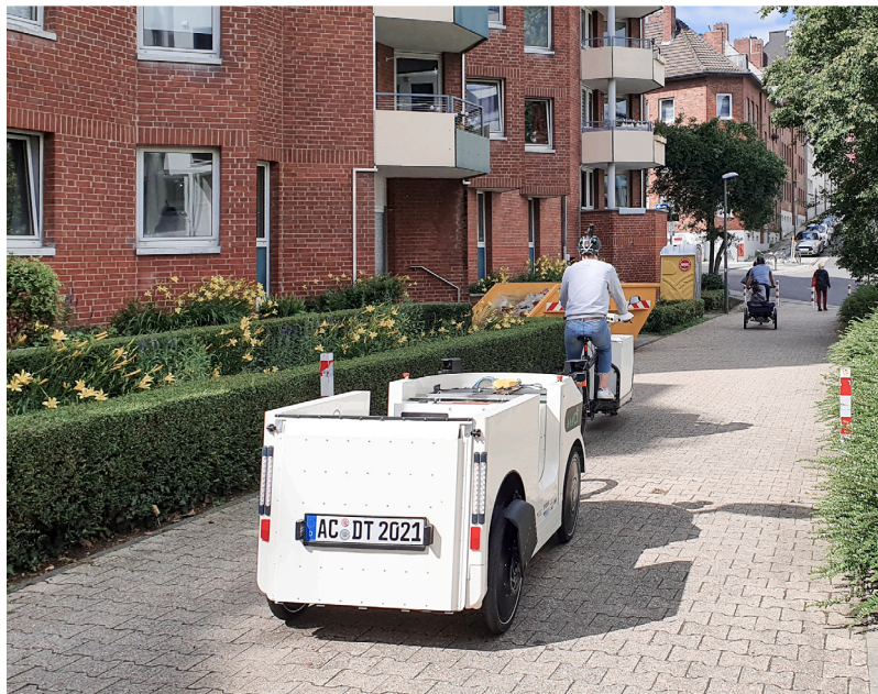
Fig. 2. A Trailer-Duck during a test ride in Aachen following a cargo bike.
