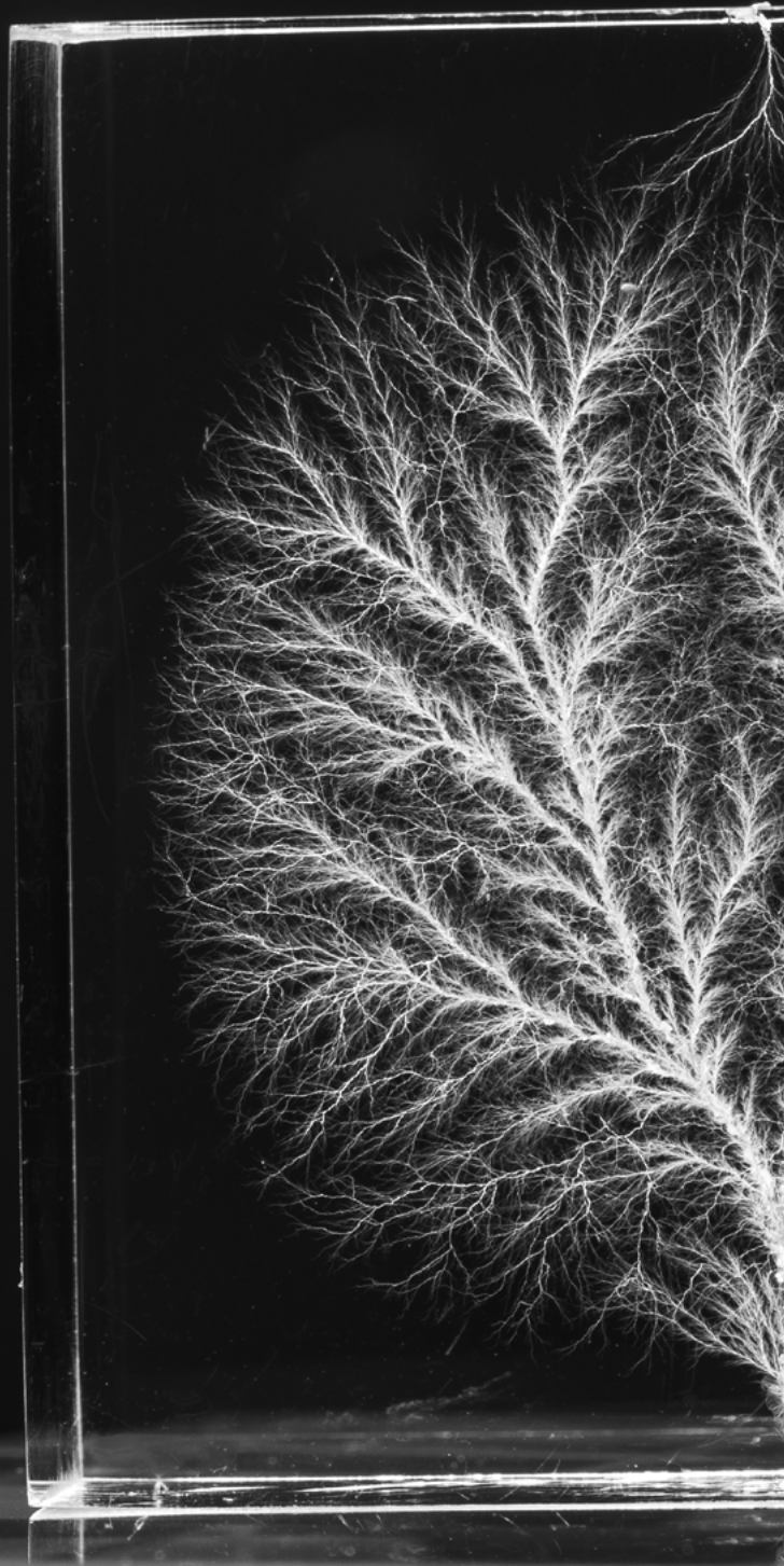
3 First vascular structures generated by partial discharge of a PMMA block initially irradiated via a 2.5MeV electron beam (Source: Emile De Visscher, 2020)
