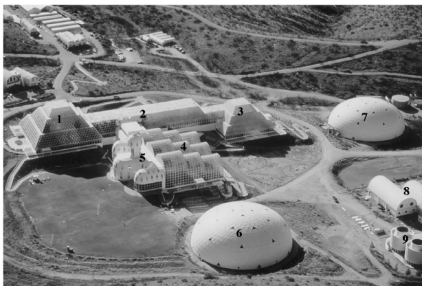
[Fig. 1] An overview of the biospheric architecture: (1) rainforest; (2) savannah/ocean/marsh; (3) desert; (4) intensive agriculture; (5) habitat; (7) south lung; (8) energy center; (9) cooling towers (Source: Dempster 1999, 34)
