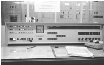
Fig. 1. The operator's interface. Computer SEL ER56 at Computing Centre, University of Stuttgart 1965. We see dials (lower right) and push buttons to get at specified data. Through the glass in the background some of the hardware
