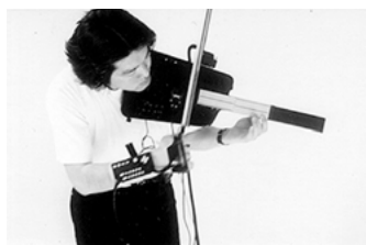
Fig. 2. The Virtual Violin, the "SuperPolm," is based upon the idea of short-range motion capture, such as finger, hand and arm movements.
