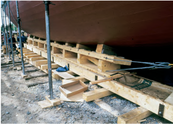
Fig. 55 The wooden tracks and sledges of a reconstruction of Jakobstads Wapen , launched in 1994 in Jakobstad. A ketch ( galeas ) with this name dating from 1767 was the first to be built and sail from the town after the partial abolishment of the Bothnian Trade Compulsion. The design was that of F.H. Chapman.
