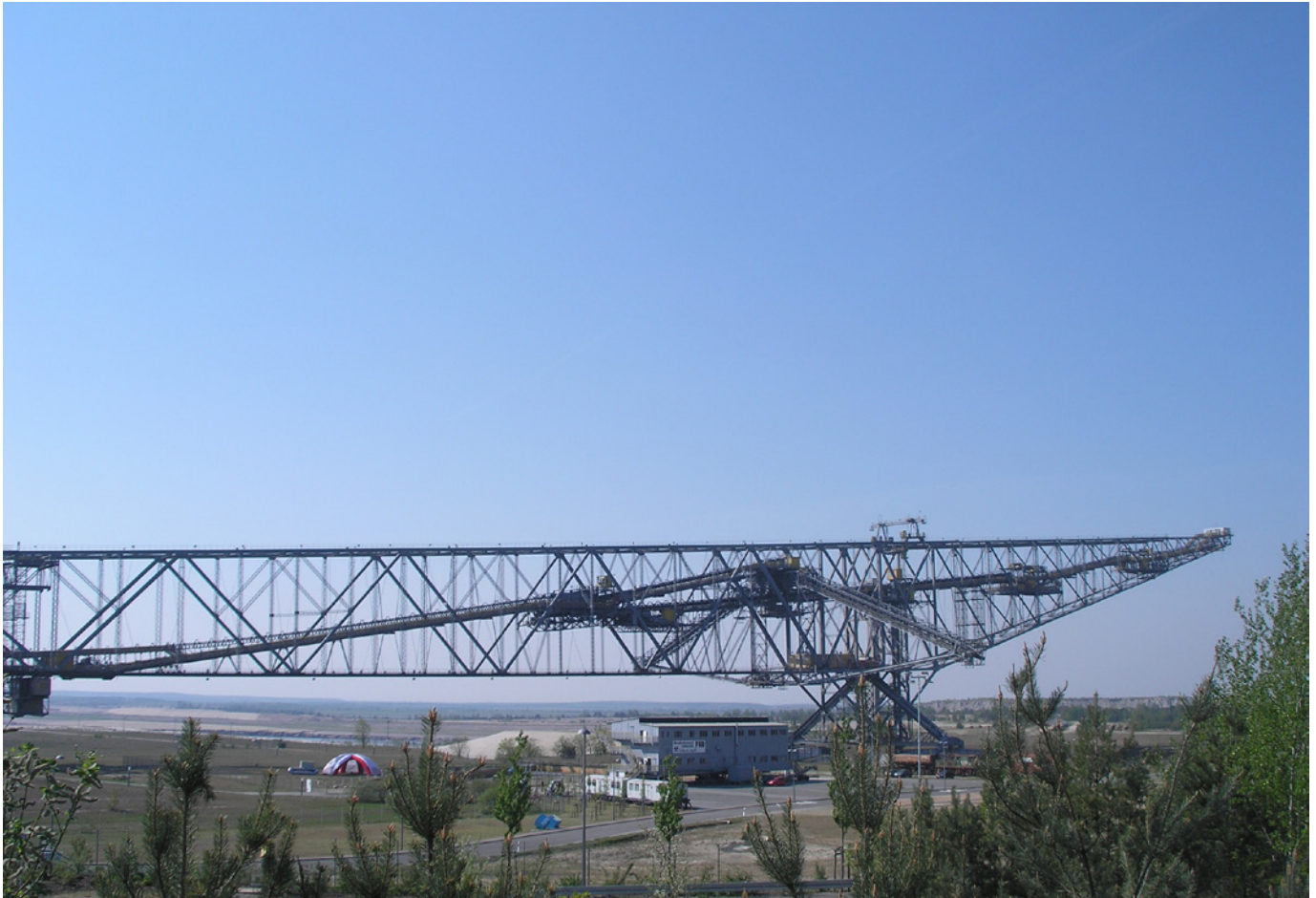
Fig. 5: The old conveyor-bridge in the mine Klettwitz: the “lying Eiffel Tower” (Deshaies 2013)
