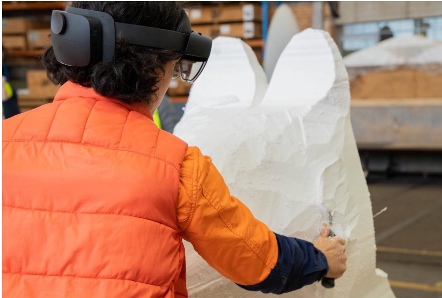
Figure 5. Using AR to sculpt forms for casting. Photo courtesy of the ARM Hub.
