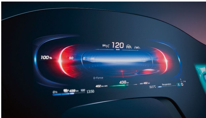
Figure 4: The Hyperscreen visualizing new kinds of driving data (electric vehicle energy “boost” and “recuperation”) using a novel “clasp”-style display
