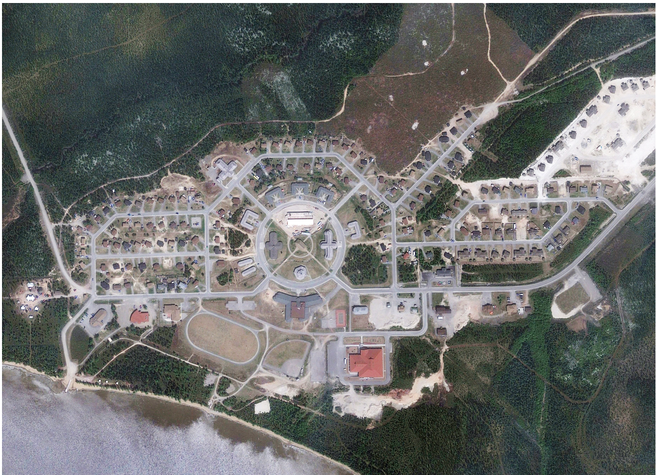
Figure 3. Oujé-Bougoumou, Quebec. Radial grid formed in the development of the new Oujé-Bougoumou community. Source: Author with base from Google Earth.
